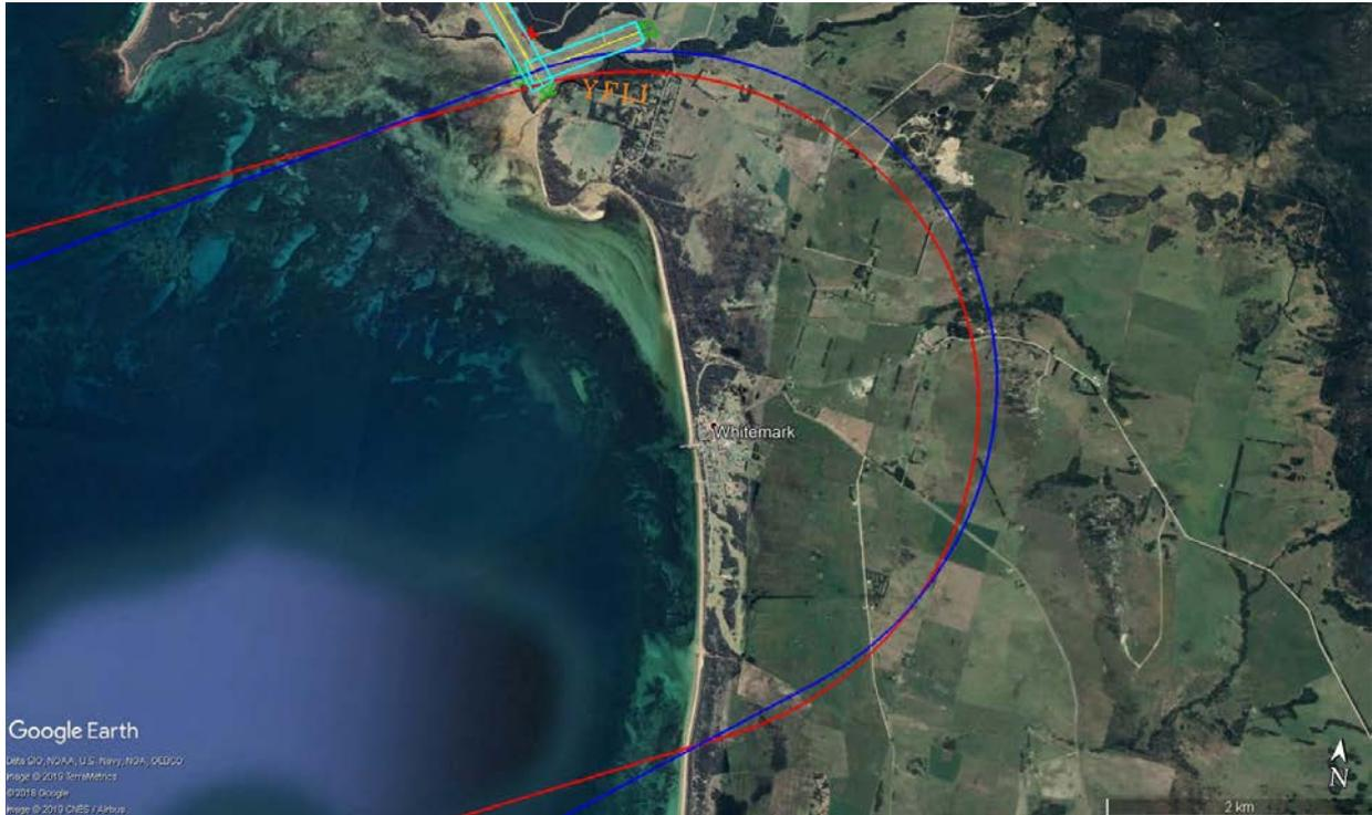
**Figure 2: Proposed amended procedure for missed approaches to Runway 05 at Flinders Island Airport**
